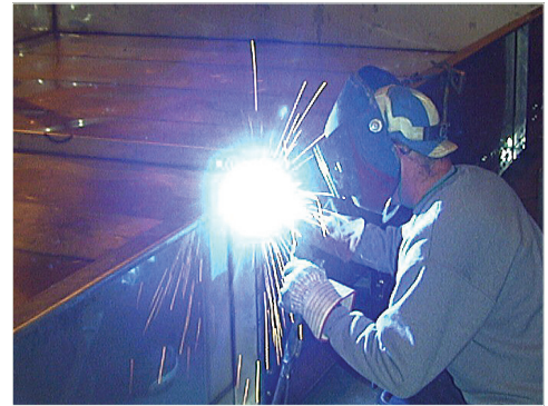
Welded Type 304 Stainless Steel Cold Water Basin
