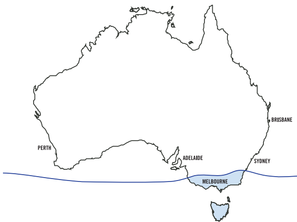
Climate Limitation of CO 2 Systems with Air Cooled Condensers
