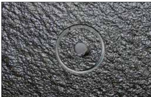
Figure 15. Scored TriArmor® Corrosion Protection System
