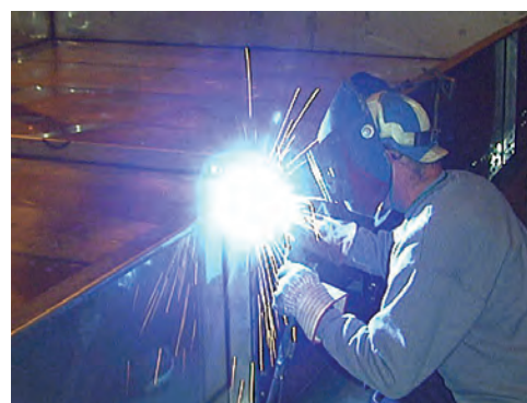
Welded Stainless Steel Cold Water Basin
