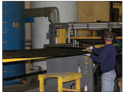
BACross® Fill Manufacturing
