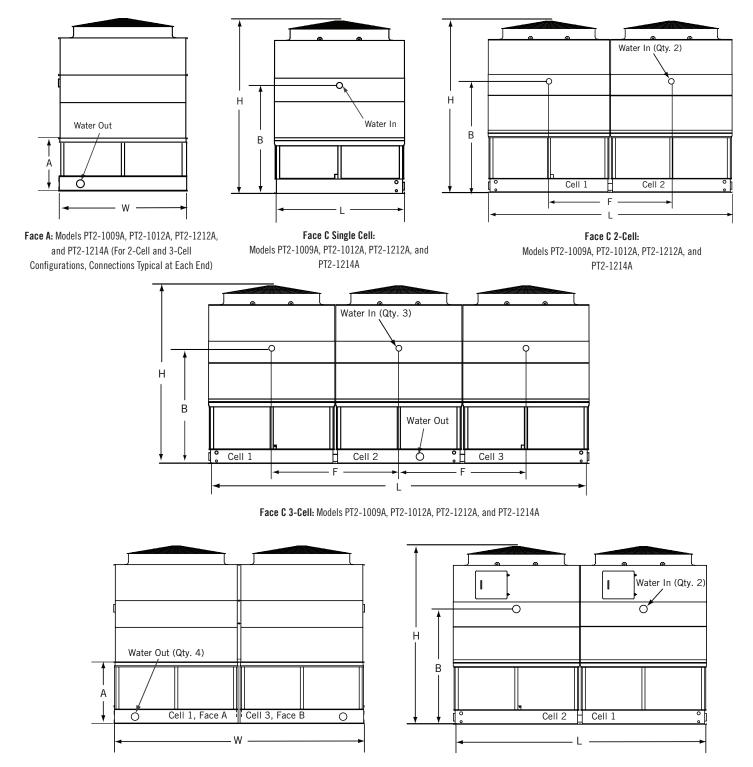
Face A/B Quad Configuration: Models PT2-1009A, PT2-1012A, PT2-1212A, and PT2-1214A Connections Typical at Each End
