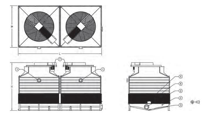
1. Water Inlet; 2. Water Outlet; 3. Drain; 4. Overflow; 5. Quick-Fill; 6. Make-Up; 7. Fan Motor.
