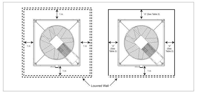
To satisfy air inlet requirements when a counter flow product is located in a louvred enclosure
