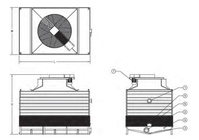
1. Water Inlet; 2. Water Outlet; 3. Drain; 4. Overflow; 5. Quick-Fill; 6. Make-Up; 7. Fan Motor.
