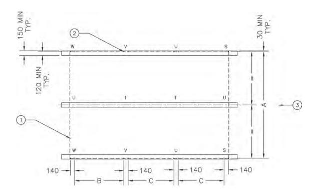
1. Outline of Unit; 2. Mounting holes; 3. Water Outlet Side; 4. Piers Can Be Offered.
