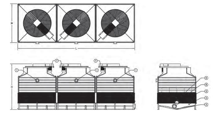
1. Water Inlet; 2. Water Outlet; 3. Drain; 4. Overflow; 5. Quick-Fill; 6. Make-Up; 7. Fan Motor.
