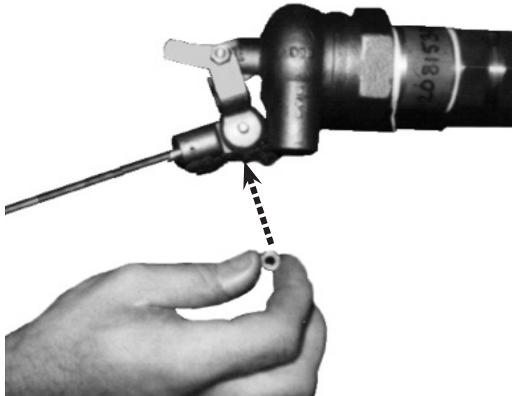
Figure 8. Attaching float arm
